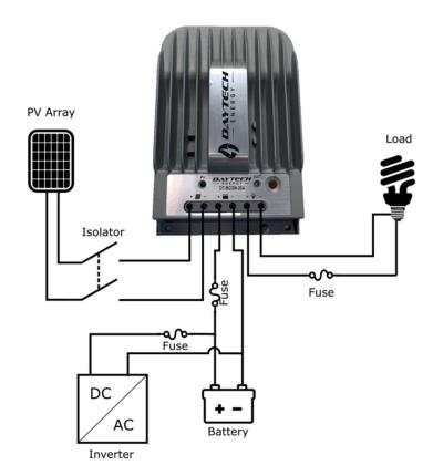
**WARNING:** Risk of electric shock. Exercise caution when handling solar wiring. The open circuit voltage of a PV array in direct sunlight can exceed 100V.
